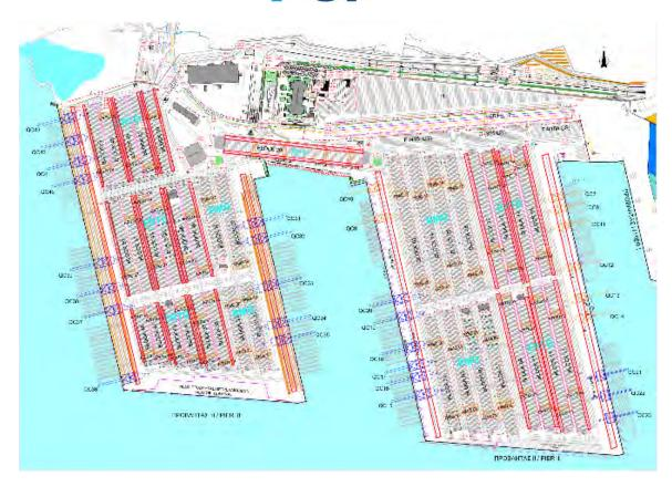
5) RTGC Operation Vehicle Quantity Inspection: When the number of vehicles waiting in the same RTGC or QC area (or other area determined from PCT user) exceeds a specified threshold (configurable), an alarm is generated and reported. The required coverage area is marked in red, while wherever possible PCT may decide to include more areas with this function with the project cameras that will be installed if available license and system resources meet minimum requirements.
