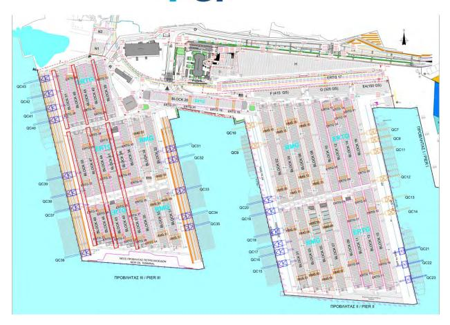
4) RTGC & QC Runway Stop Detection: If a vehicle is parked on the track of port machinery such as RTGC or QC (or other area determined from PCT user) for more than a predetermined time set by PCT user (i.e. 30 seconds), an alarm is generated and reported. The required coverage area is marked in red, while wherever possible PCT may decide to include more areas with this function with the project cameras that will be installed if available license and system resources meet minimum requirements.
