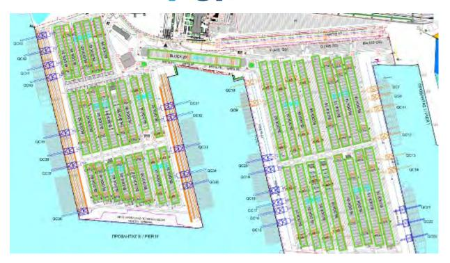
8) Virtual Fencing: If a person is detected in the perimeter area of the wharf (or other area determined from PCT user), an alarm is generated and reported. The required coverage area is marked in blue, while wherever possible PCT may decide to include more areas with this function with the project cameras that will be installed if available license and system resources meet minimum requirements. The Virtual Fencing will be applied also at all PCT perimeter borders to enforce security.
